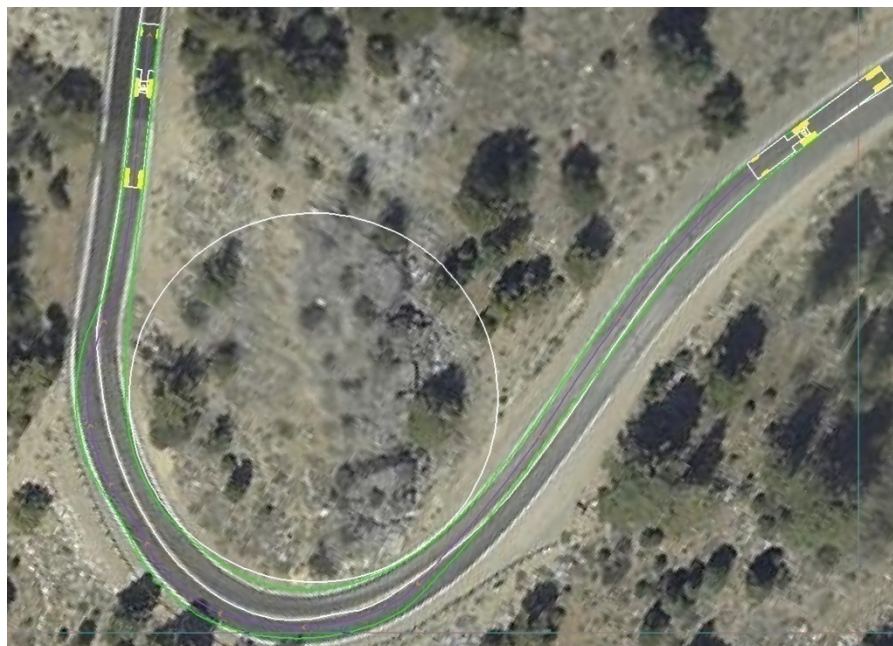
MNO 108 – Example of Truck Off-Tracking at PM 7.0
