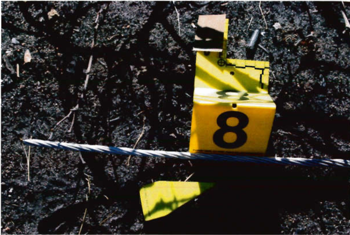
P-KG-315 8d - Power line section, end 6 close up
