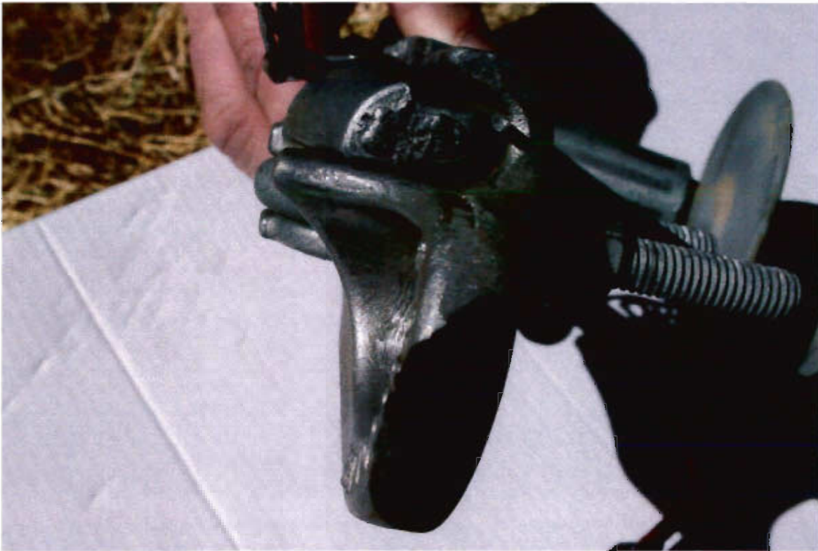
P-KG-283 8a - Close up of wire shoe with piece of power line attached
