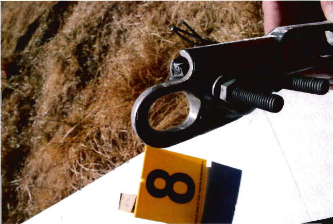
P-KG-285 8a - Close up of wire shoe with piece of power line attached
