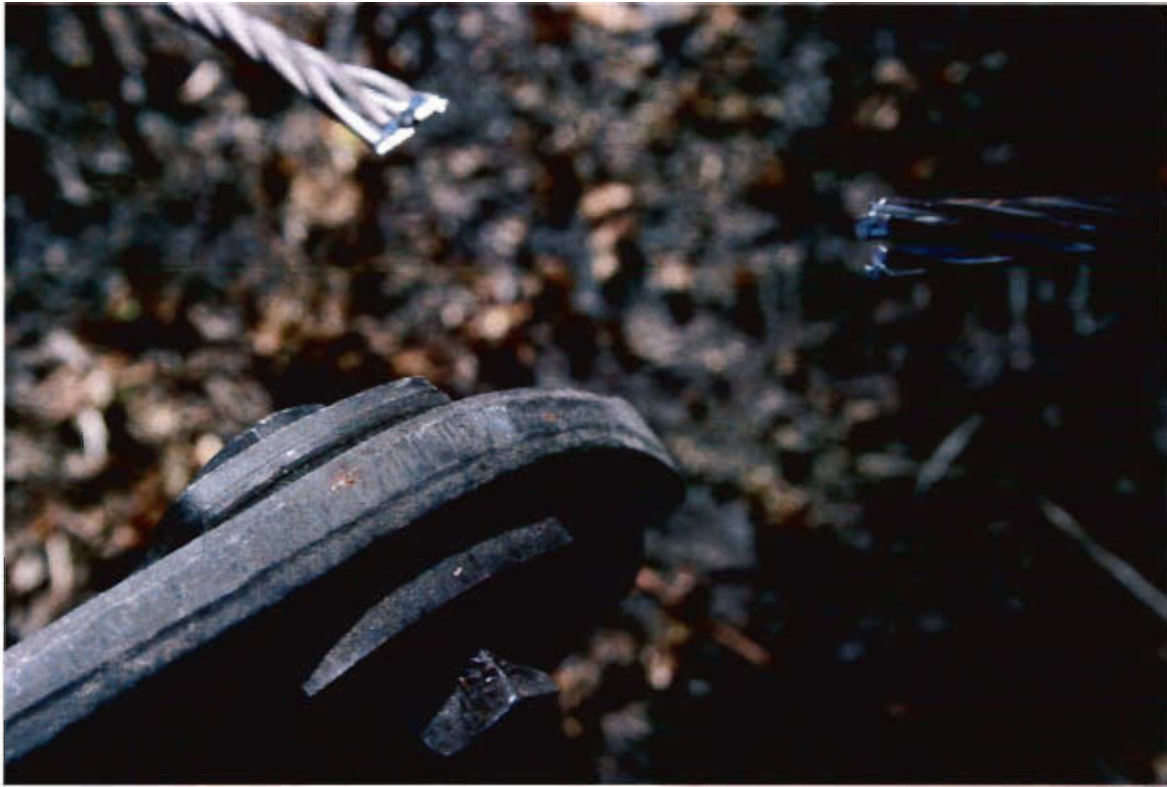
P-KG-319 9a - Cut power line
