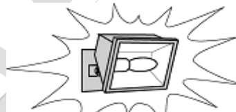
Glare from unshielded floodlight
