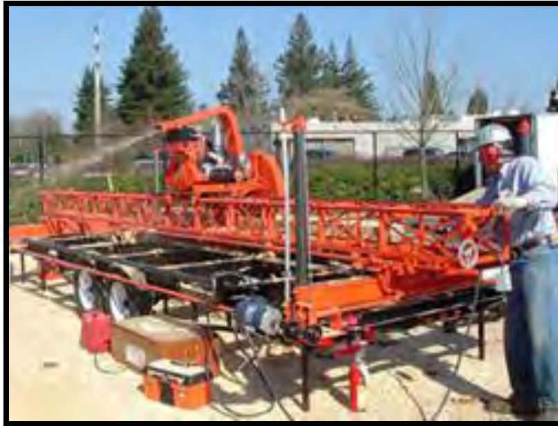
Figure 17. Mobile Dimension Sawmill
